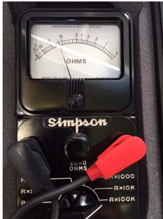
Simpson 372 ohmmeter (45-VDC) showing 1.2 mohms leakage to ground on a sensor cable.
