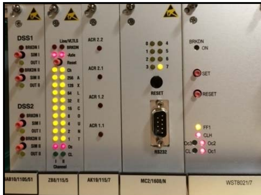
Fig. 17: Minus axle LED status indication. Note that the vertical column of LEDs would be flashing alternately
