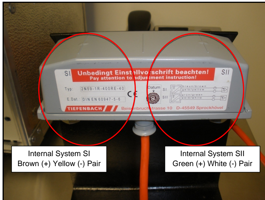
Fig. 4: Structure of DSS showing internal systems one and two
