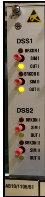
Fig.13: Metallic Object or Wheel Flange Resting Atop Both Systems of the Sensor
