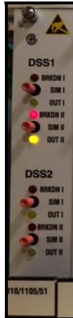
Fig. 11: Amplifier card front panel indicating DSS 1 SII shorted or open cable. Note both yellow “OUT” and red “BKN” LEDs illuminated.
