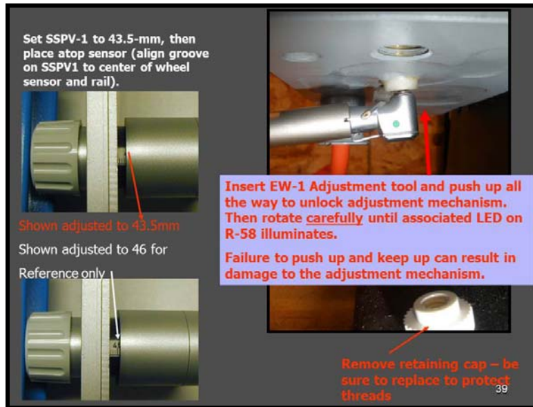
Fig 7: Illustration showing SSPV-1 set to 43.5-mm, and EW-1.
