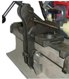
Illustration 15: Attach fastening arm DBG-F to the distance gauge
