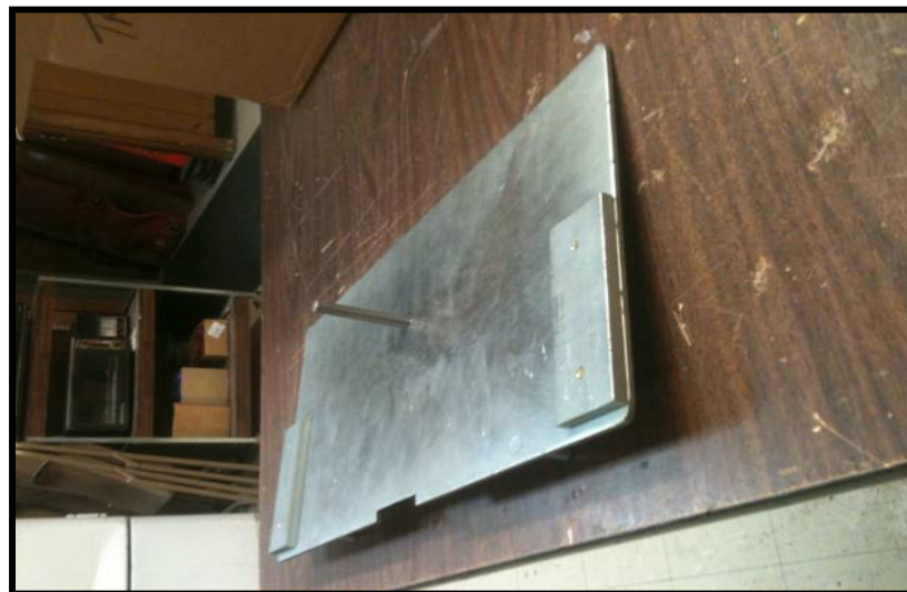
Fig.8: An unauthorized “test” plate provided by a manufacturer of defect detectors and AEI scanners.
