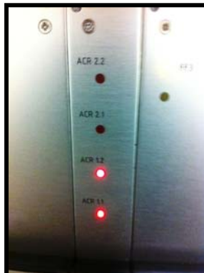
Fig. 24: AK19 module assigned to one Binary Counter Module with channels 1.1 and 1.2 activated. Both LEDs within the pair should illuminate when the ACR key is actuated.
