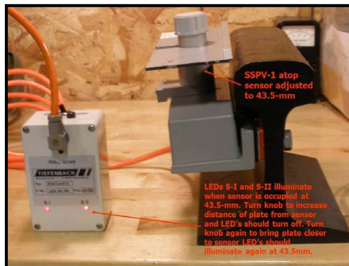
Fig. 6: R-58/117/1 Device showing S1 and S2 LEDs illuminated when SSPV-1 Plate is at 43.5-mm.
